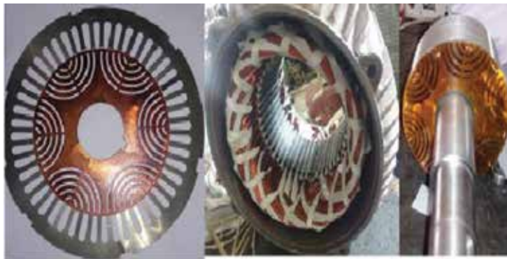
Figure 12. Fabrication details of 8-6-4 BDFRM.
