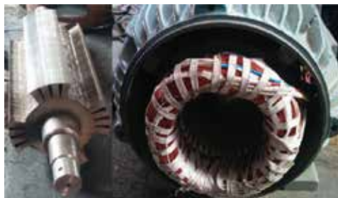
Figure 11. Fabrication details of 6-4-2 BDFRM.
